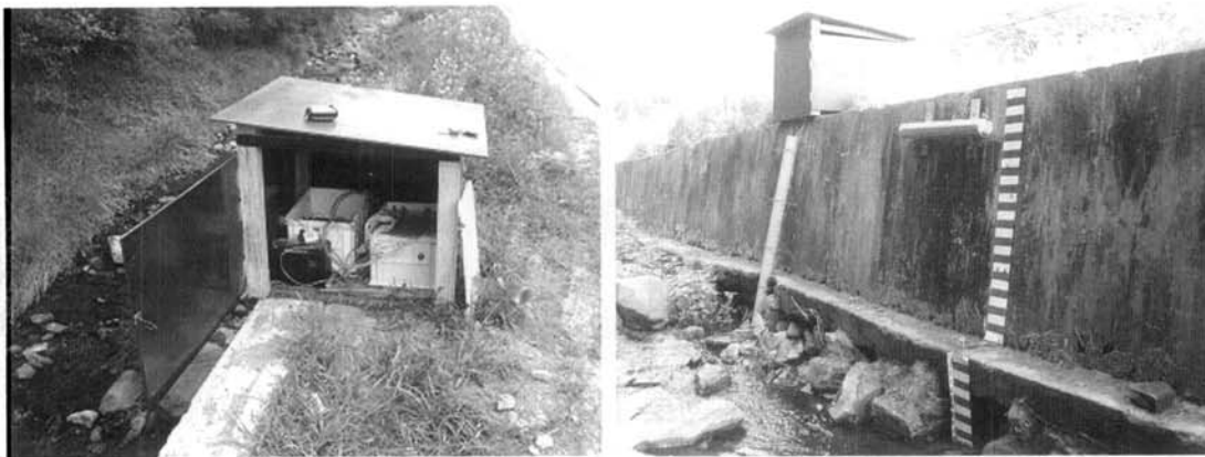
Fig. 4. Flow and automatic water sampler installed at the outlet of Wolgok-ri watershed.
